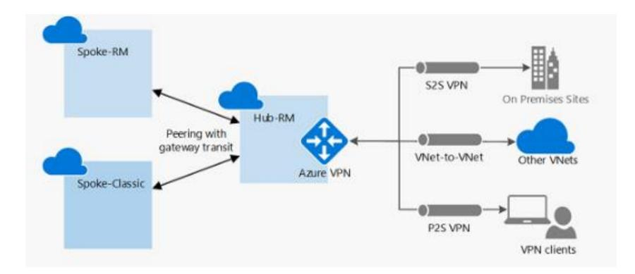
In the diagram, gateway transit allows the peered virtual networks to use the Azure VPN gateway in Hub-RM. Connectivity available on the VPN gateway, including S2S, P2S, and VNet-to-VNet connections, applies to all three virtual networks.
